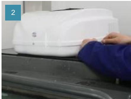
2. Place the Skimo A/C unit on the roof. Fasten it from the inside of the cabin with the 4 M8 screws and their washers removed in section 7.3-preparation of the Skimo A/C unit
