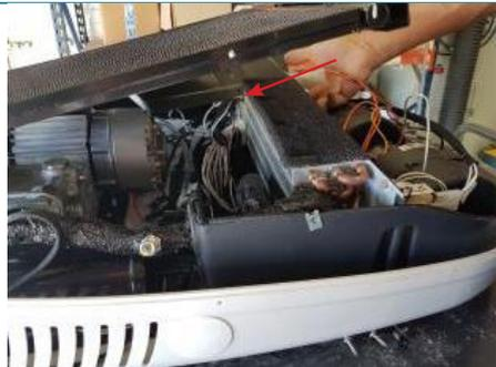
5. Lift the evaporator by taking it on the opposite side of the thermostat.
