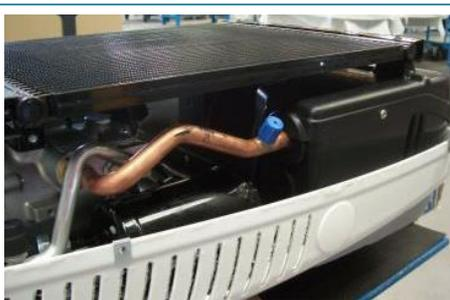
9. Reassemble the evaporator block cover and the condenser assembly with the original screws.
