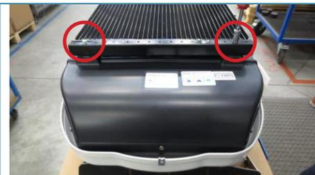
1. Remove the white top cover and unscrew the 2 screws fixing the front of the condenser.
