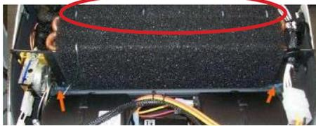
6. Remove the bulpren holding hooks on the upper side of the evaporator. Remove the bulpren by removing it from underneath the evaporator.
