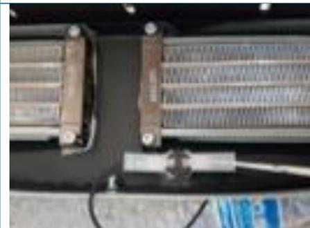
4. Connect the safety heat resistors.
