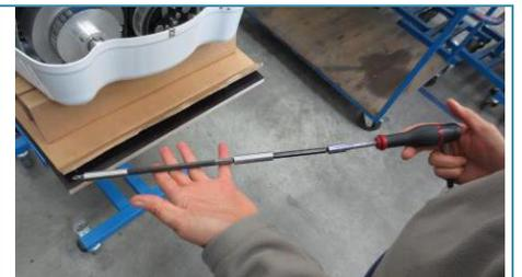
3. For the sixth screw at the back of the lid, lengthen the screwdriver.
