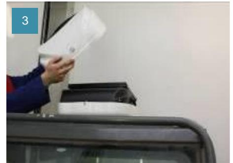
3. Remove Skimo A/C unit cover: remove its 6 fastening screws and unplug the ventilator connector.
